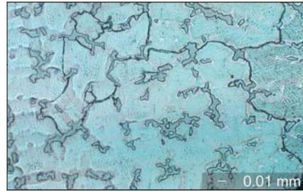
All ReCap™ M<sup>2</sup>a™ resurfacing components possess a high carbon, high carbide (> 20% carbide content) microstructure with “blocky” carbides resulting from “as cast” vacuum processed raw material.
